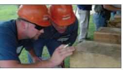
...and everyone is supposed to be 100 percent on the question of whether the test ties are grade ties or are to be rejected for defect.
